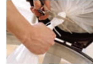
Seamless bag system prevents dust leaks when changing.
